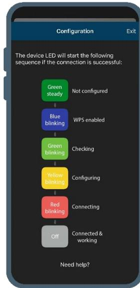
Figure 24.- Lighting Wi-Fi Configuration sequence WPS mode.
