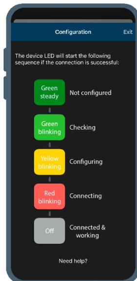
Figure 18.- Lighting Wi-Fi Configuration sequence.
