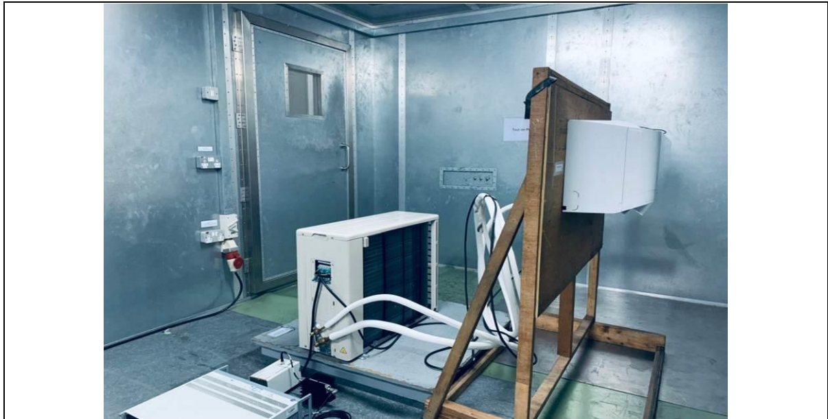
Figure AIII.5: Injection current test set-up
