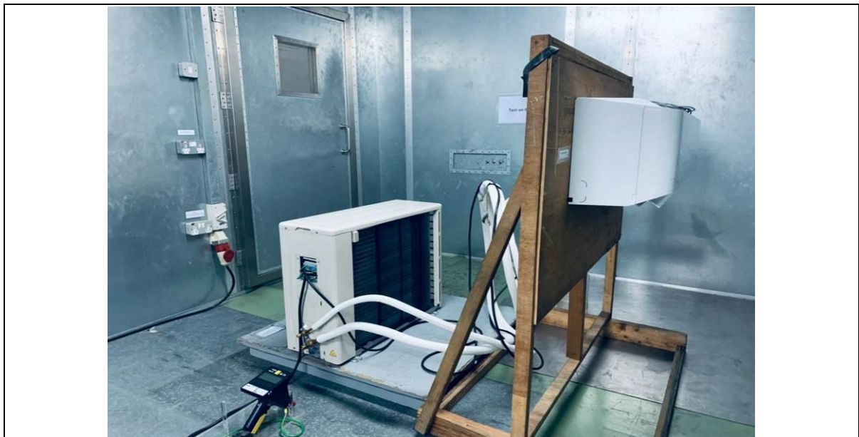
Figure AIII.4: Electrostatic discharge test set-up
