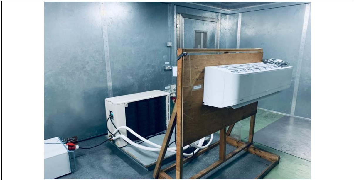
Figure AIII.1: Continuous/Discontinuous disturbance voltage test set-up
